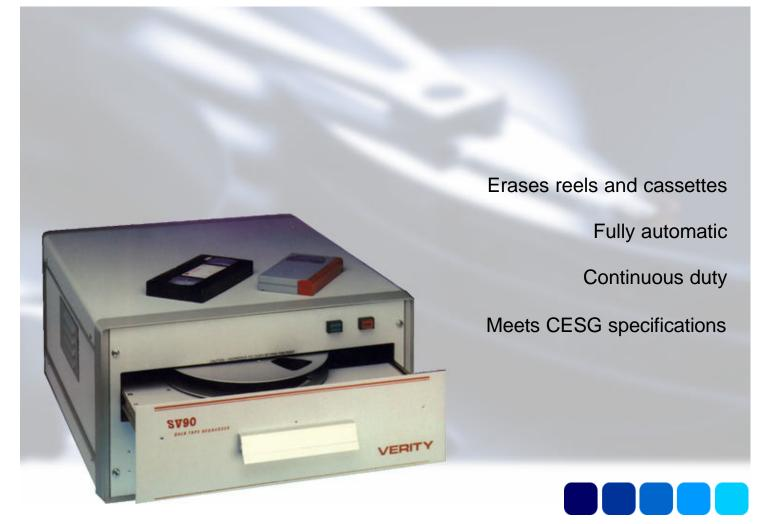
The SV90 is able to perform automatic erasure of high-density magnetic media achieved by applying a highly focused magnetic field created by Verity Systems exclusive multi-axis, 'pole tip' design. The tapes or cassettes are placed in the draw compartment and rotated within the powerful 7000 Gauss field ensuring uniform and complete erasure.
