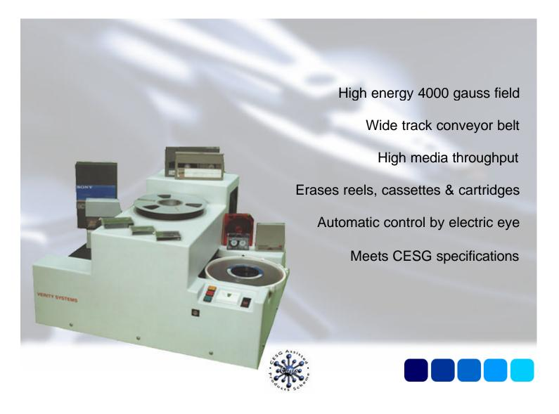
The performance of the SV5000 will satisfy requirements for volume erasure of high-density metal tapes and cassettes. Automatically controlled by an electric eye, the reels, disks or cassettes are placed onto the wide conveyor belt where they are transported through the 4000 Gauss field. Up to five thousand diskettes or five hundred cassettes or cartridges can be erased per hour.
