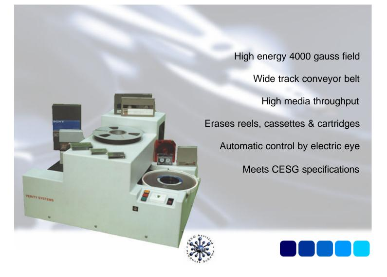
The performance of the SV5000 will satisfy requirements for volume erasure of high-density metal tapes and cassettes. Automatically controlled by an electric eye, the reels, disks or cassettes are placed onto the wide conveyor belt where they are transported through the 4000 Gauss field. Up to five thousand diskettes or five hundred cassettes or cartridges can be erased per hour.
